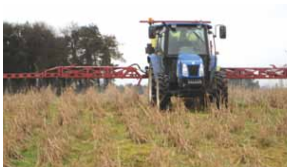
Miscanthus is sprayed with glyphosate at 4 litres per ha to eliminate grass weed while the miscanthus is dormant.
